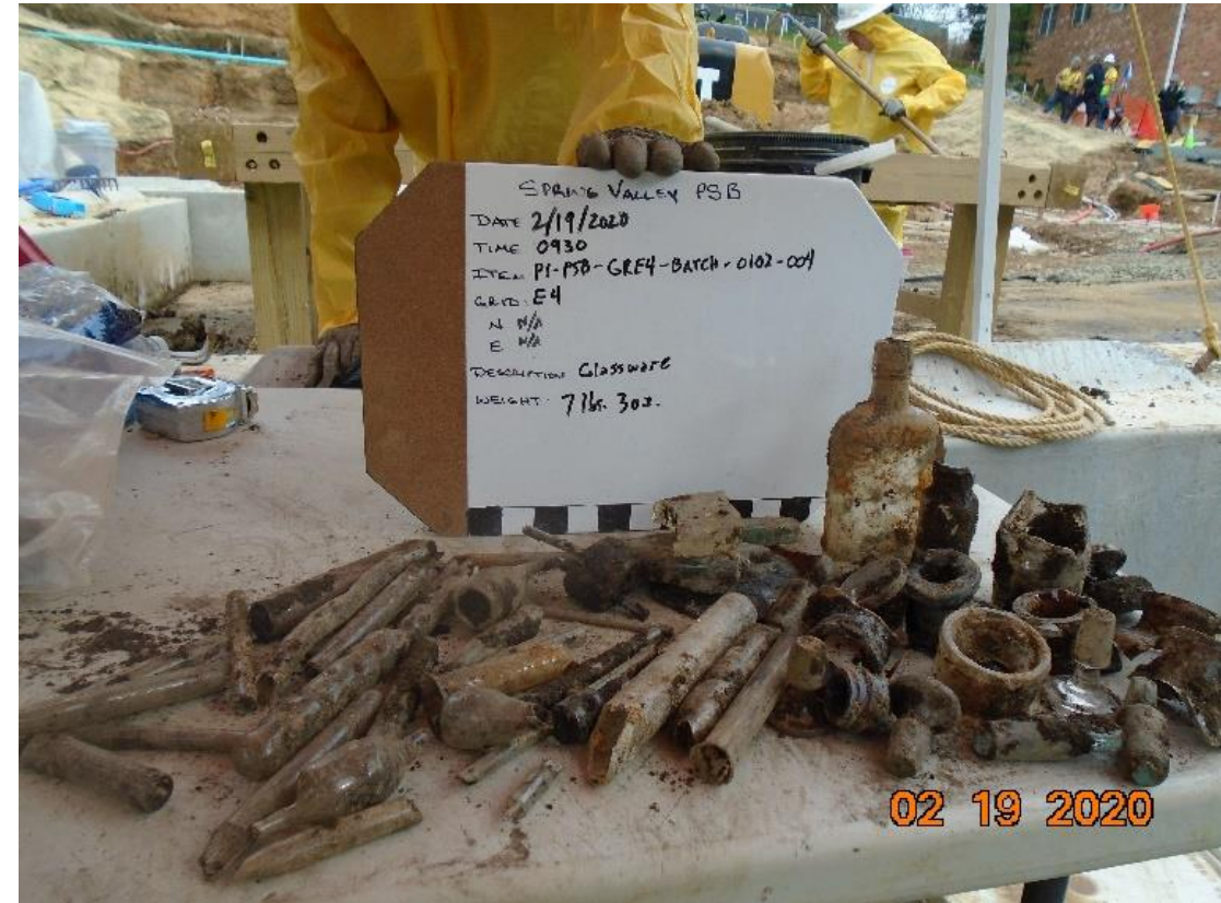
Examples of AUES Debris recovered: broken glass, glass jars, test tubes, ceramics, and metal pieces. No CWA was detected. One area had elevated metals in the soil and one test tube was found with possible TNT - both were removed.
